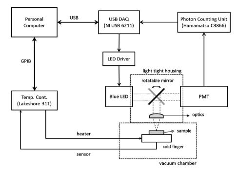
Figure 1. Simplified block diagram of the TL measurement set-up.
