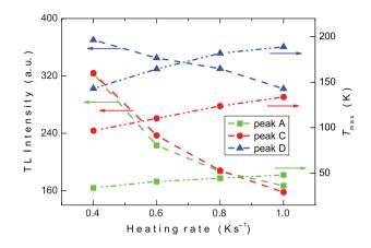
Figure 4. (colour online) Heating rate dependencies of TL intensities and peak maximum temperatures.
